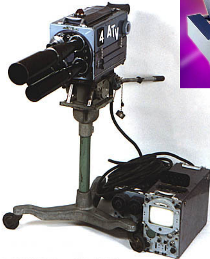
1952 Pye Mark-III (UK) Image Orthicon 405-line TV Co
